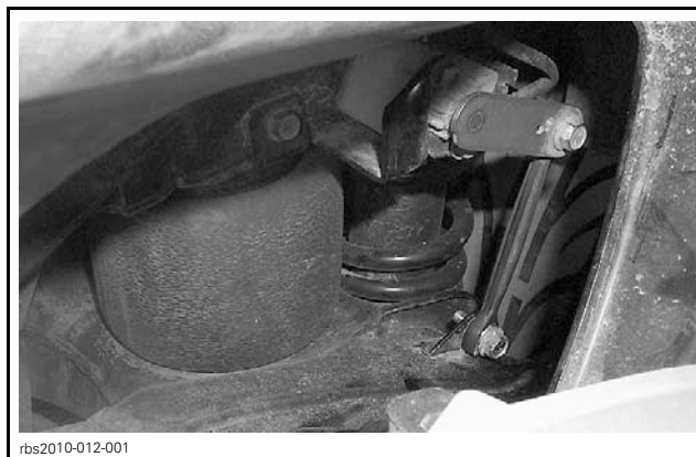
ACS LEVER – CORRECT ORIENTATION
