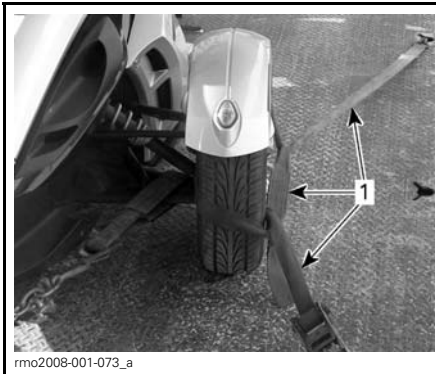
rmo2008-001-073_a TYPICAL FRONT WHEELS ATTACHMENT — METHOD 2
