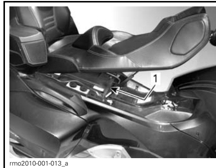
1. Fuse box located under the seat
