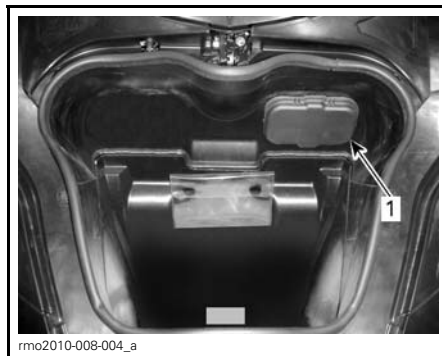
TYPICAL 1. Fuse box in front storage compartment
