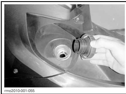
FUEL CAP ON LEFT SIDE UNDERNEATH SEAT
