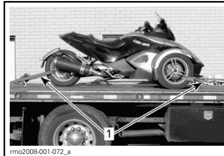
rmo2008-001-072_a TYPICAL 1. Front and rear wheel firmly attached to trailer
